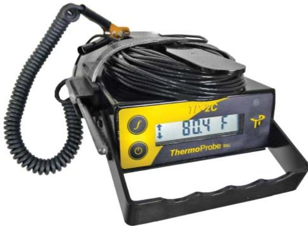
The TP2 of the early 1980s became a long time favorite of many petroleum inspectors. It was the first portable electronic thermometer, PET, to challenge the long reign of the cup case thermometer. Although the TP2 was severely dated by 1990, many inspectors wanted nothing else despite newer models by ThermoProbe and various competitors. Because the US market demanded the return of the venerable black box, ThermoProbe has put its newest circuit and software design into the old familiar form.
